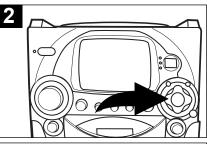
During playback, press the Skip/Search (◄◄) button once to move the player back to the beginning of the current track. Press the Skip/Search (◄◄) button repeatedly to move the player back to lower numbered tracks.
